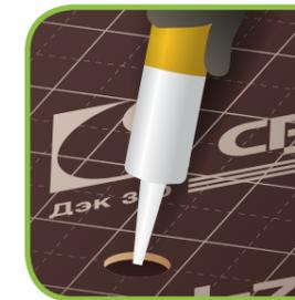
Fill all holes, made in the course of installation works, with a silicone-based adhesive to prevent penetration of moisture (swelling).
