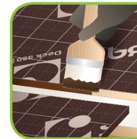
When cutting plywood, protect flat ends with paint, such as Teknol JRL (Finland), or a sealant to prevent penetration of moisture (swelling).
